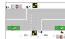
Example 2 - measurement of distance - children's crossing with 2 parallel continuous or broken lines
